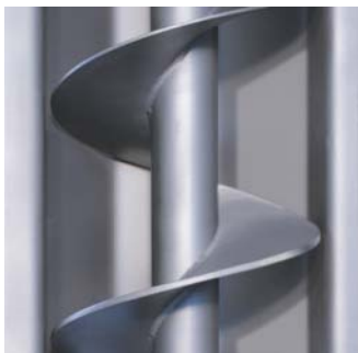
Vertical feedscrew transfers product without smearing
